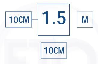
These markings should be in red or alternatively a colour which contrasts sharply with the paving/surround. Depth markings should be placed at regular intervals. Minimum 2m apart on small pools, 3m apart on large pools. (Small pools = less than 6m square and Large pools = more than 6m square). Depth markings that are painted should not be allowed to fade. It is recommended that they are repainted/retouched every month.
